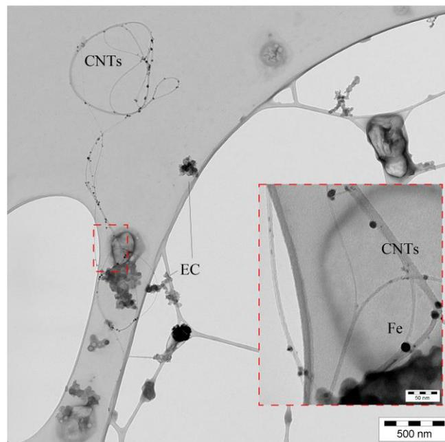
Figure 2 TEM image of CNTs collected in workplace air under normal operating conditions.
