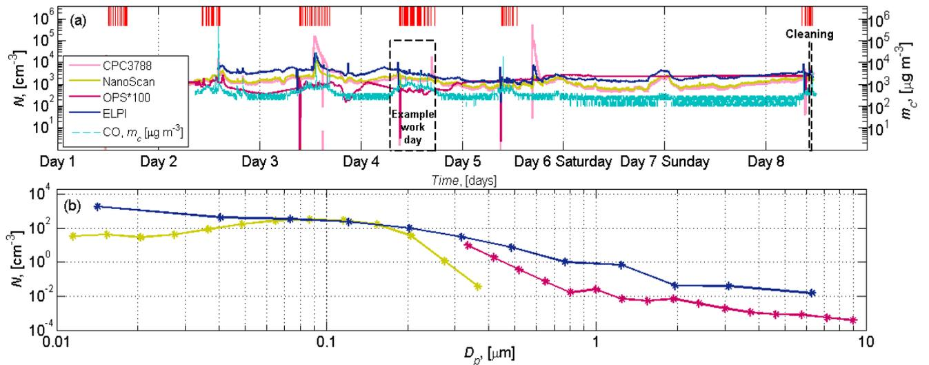
Figure 1 (a) Time series of particle number and CO concentrations and (b) particle number size distributions measured by ELPI, NanoScan and OPS with corresponding color line in (a). The red vertical lines in (a) correspond to reactor opening times when the expected CNTs emissions may occur.
